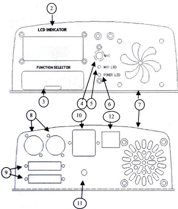
1. Laser Emitting      2. LCD Indicator for working mode      3. Function Selector      4. Sound Active Microphone
